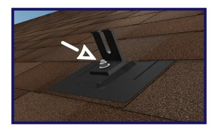
Secure the bracket to the stud using the serrated flange nut and torque to 50-inch pounds.
